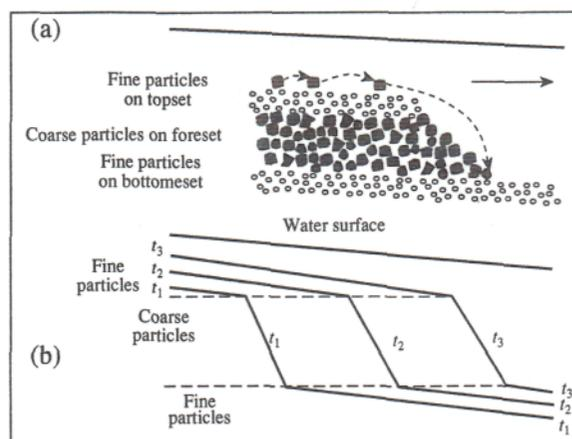
Fig. 3. Results of experiments. (a) Schematic formation of graded beds. (b) Time sequence of deposit formation for  $t_1 < t_2 < t_3$ .
